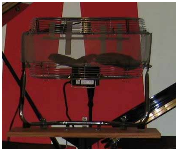
Figure 6—Propellor mechanism installed on 18-inch industrial fan
