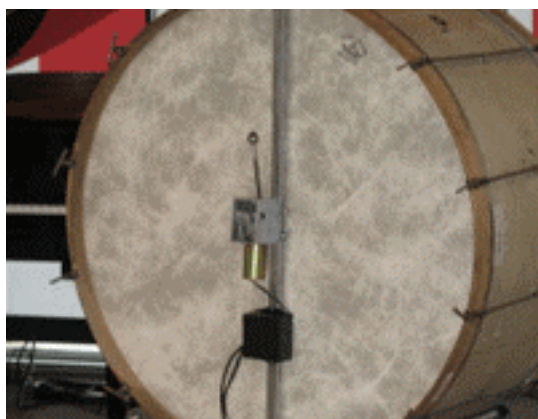
Figure 3—Bass drum with BeaterBot
