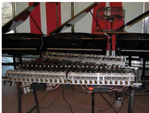
Figure 5—XyloBot mechanisms on a concert xylophone. Propellor mechanism is in the background.
